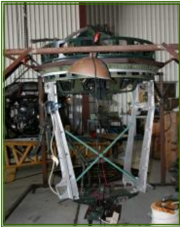
One of the few Top Turrets in the world being prepared for installation.
