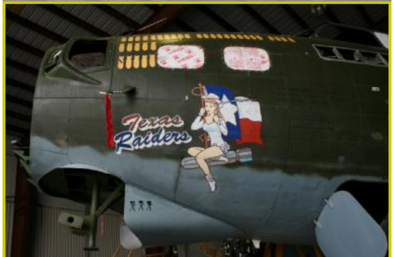
New Plexiglas, clean paint and crevices ready for attachments. Texas Raiders is being prepared for an award winning Reveal.
