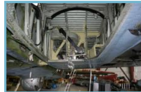
Underside view of left wing cavity, demonstrating the in-depth cleaning.
