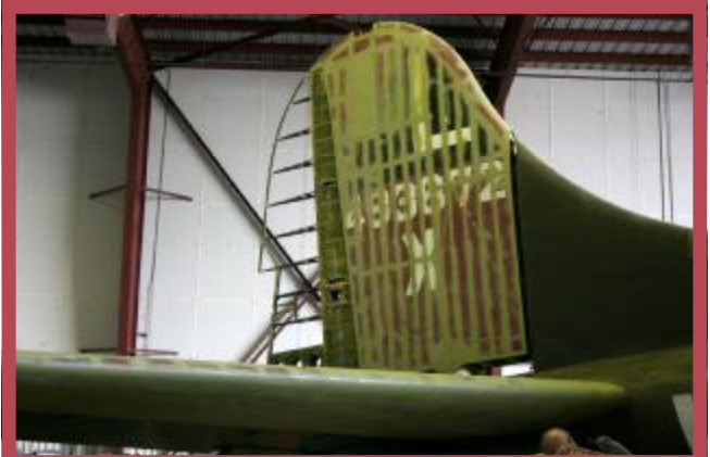
Adjuster Bars now present on the trim-tab of TR's Rudder.
