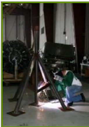
Col Tom Taylor, welding a support stand for TR. Photo by Col S Thompson
